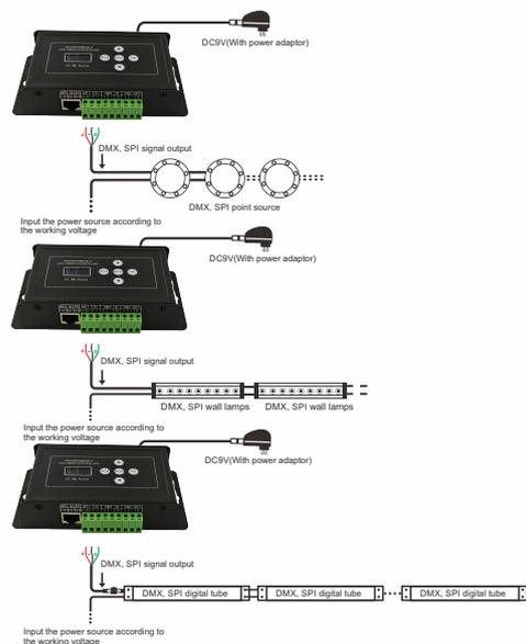
2) Pixel light controller connect to DMX decoder:
