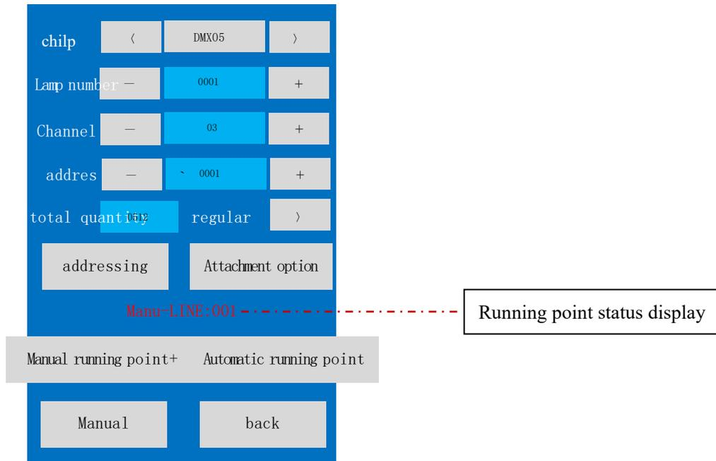
Chip: by default, DMX05, can switch and select the corresponding chip according to the "<" >" two buttons. MR-DMX05,,UCS512C,UCS512D/E/F,SM16512,TM512,SM17500, and other DMX512 decoding chips are currently supported.
