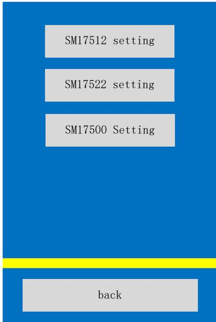
In the SM chip setting, at present, it contains the DMX512 control chip produced by SM17512, SM17522, SM17500 and other SM, in which the setting parameters mainly include the number of channels, the automatic address function turned on or off, and the setting of R/G/B/W self-check color. Channel current adjustment and other functions.
