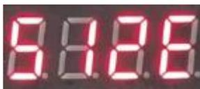
Then press MENU to n mode, set the total number of channels occupied by this transcoding chip, for example, if this chip has 16 RGB lights, it is set to 48; if it has 16 RGBW lights, it is set to 64.
